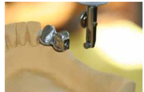
After screwing in the stud, the housing is secured in the parallel mandrel and the fit is tested.
