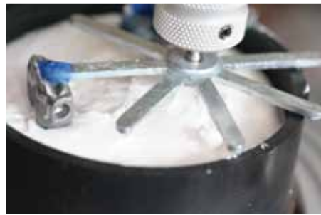
To prepare a milling model, the crowns are removed from the master model with a transfer device and placed in wet plaster after being pinned.
