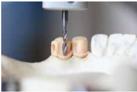
The wax miller begins cutting the lingual facing to approximately 1.5mm with a speed of 5,000 to 7,000 RPM.
