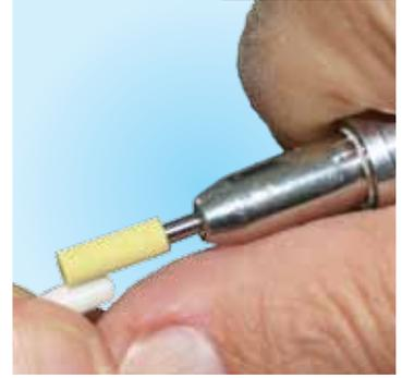
Reduce surface roughness using the new cylinder yellow diagen and other new shapes.
