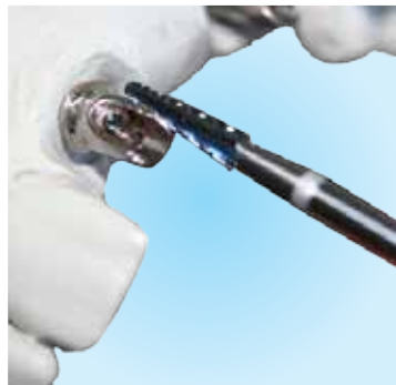
Narrow and difficult areas are approached with cutter D198KT23.
