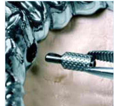
The housing is blasted with AlOx2 before the titanium pin is bonded with DTK adhesive.
