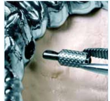
The housing is blasted with AIOx2 before the titanium pin is bonded with DTK adhesive.
