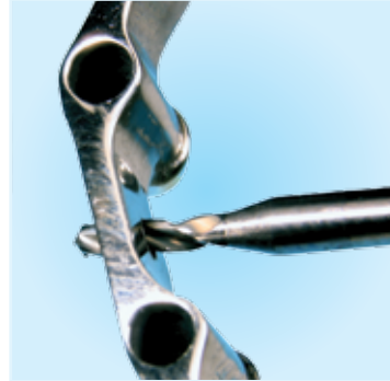
The bar is perforated with either the 1.0 mm, 1.4 mm or 1.8 mm drill to accommodate the pin.
