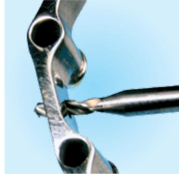
The bar is perforated with either the 1.0 mm, 1.4 mm or 1.8 mm drill to accommodate the pin.
