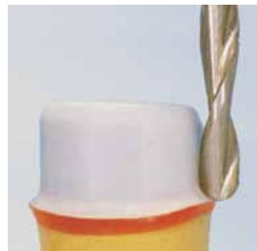
Spiral wax miller 0° with rounded end. F1352W23 at 3,000 to 5,000 rpm.
