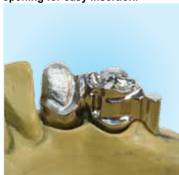
The crowns are cast and the lingual areas and male attachment are refined with milling burs.
