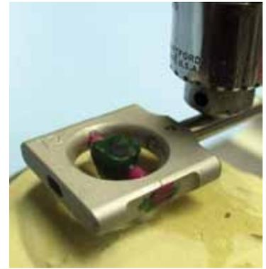
Positioning of the wax up into the cutting frame.
