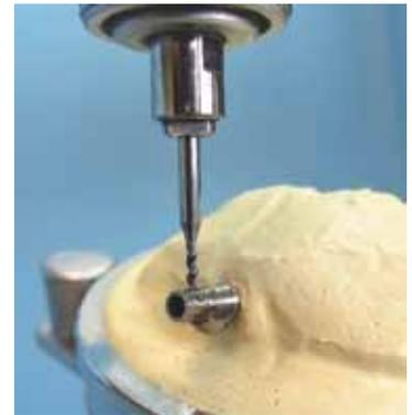
Drilling the hole before cutting the thread.
