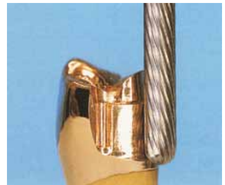
After casting & finishing, the parallel surface is remilled with profile bur, F1272H23.
