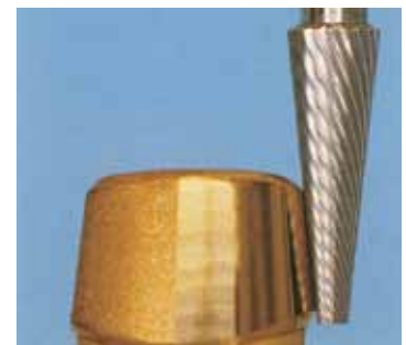
The profile milling tool finishes the surface of the 6° tapered crown precisely.
