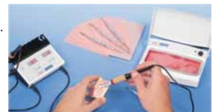
Renfert's Waxelectric and Wax Profi being utilised for faster waxing.
