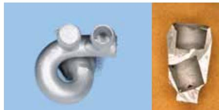
The considerable expansion of the competitor's resin during the incineration phase resulted in the fracture of the investment material die in the casting ring. After casting, the crown is sealed with a lid and can not be used.
