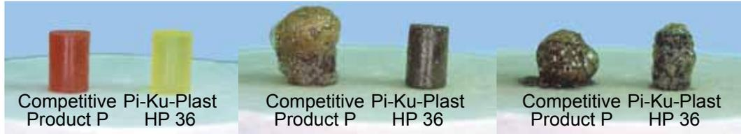
Identical blocks of the competitor's resin (left) and Pi-Ku-Plast HP36 are ready for the incineration test.
