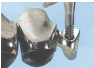
Cut the thread into the substructure. First use the first tap and then the last tap.
