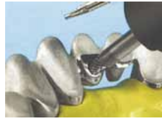
Assemble the substructure and superstructure up to the stop using the tungsten carbide facing cutter.
